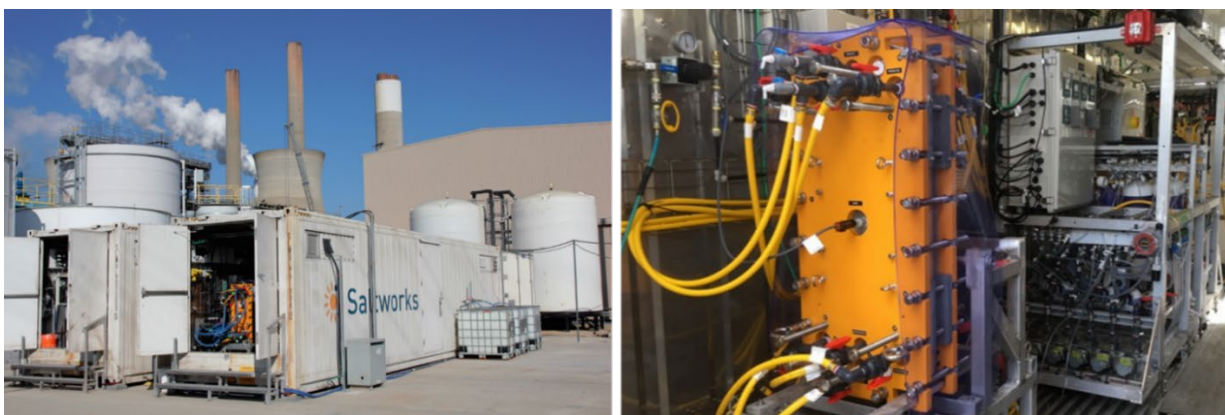
Figure 1 Flex EDR Selective Pilot Plants (left) and Flex EDR Selective Stack (right)
