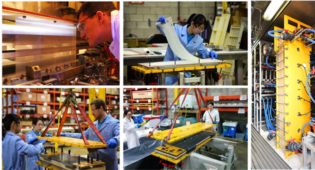
Figure 2-3 Full-Scale Production of Electro dialysis Stacks and Membrane
