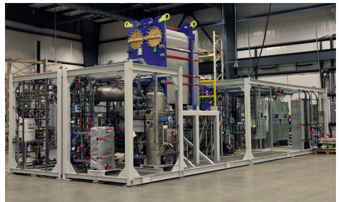
In-house assembly of a SaltMaker MVR plant
